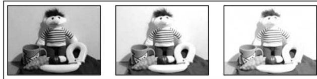
Fig. 9. Three images of a static scene taken with a Nikon 990 Coolpix camera using exposures e , 2e , and 4e (left to right). These images were used to recover the inverse response of the camera (see Fig. 10).
