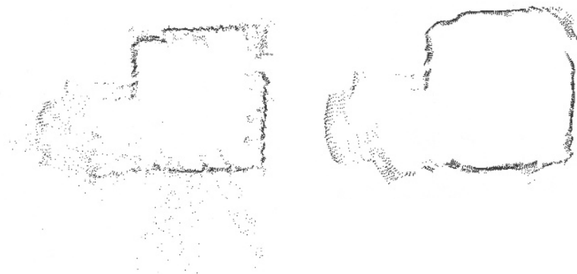
(a) After applying multibaseline stereo (b) Median-filtered version of (a)
