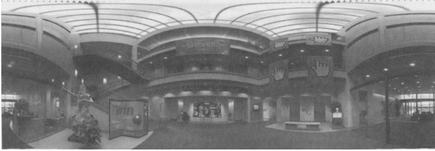
FIGURE 13.15. Tessellated spherical panorama covering the north pole (constructed from 50 images). The white triangles at the top are the parts of the texture map not covered in the 3D tessellated globe model (due to triangular elements at the poles).
