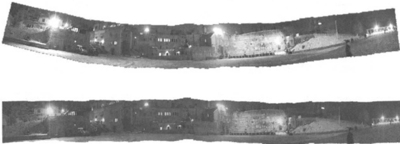
FIGURE 16.14. Mosaicing from a panning camera which is slightly tilted upward. Regular mosaicing results in a curled image, while rectified mosaicing results in a straight mosaic.
