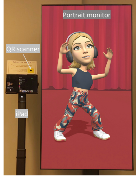
Figure 2: DanceCraft Kiosk: The kiosk features an iPad for user to play music. The avatar dances in response to the music on a life-sized portrait monitor. Users can cast their personal 3D Bitmoji by presenting a QR code to the QR code scanner.
