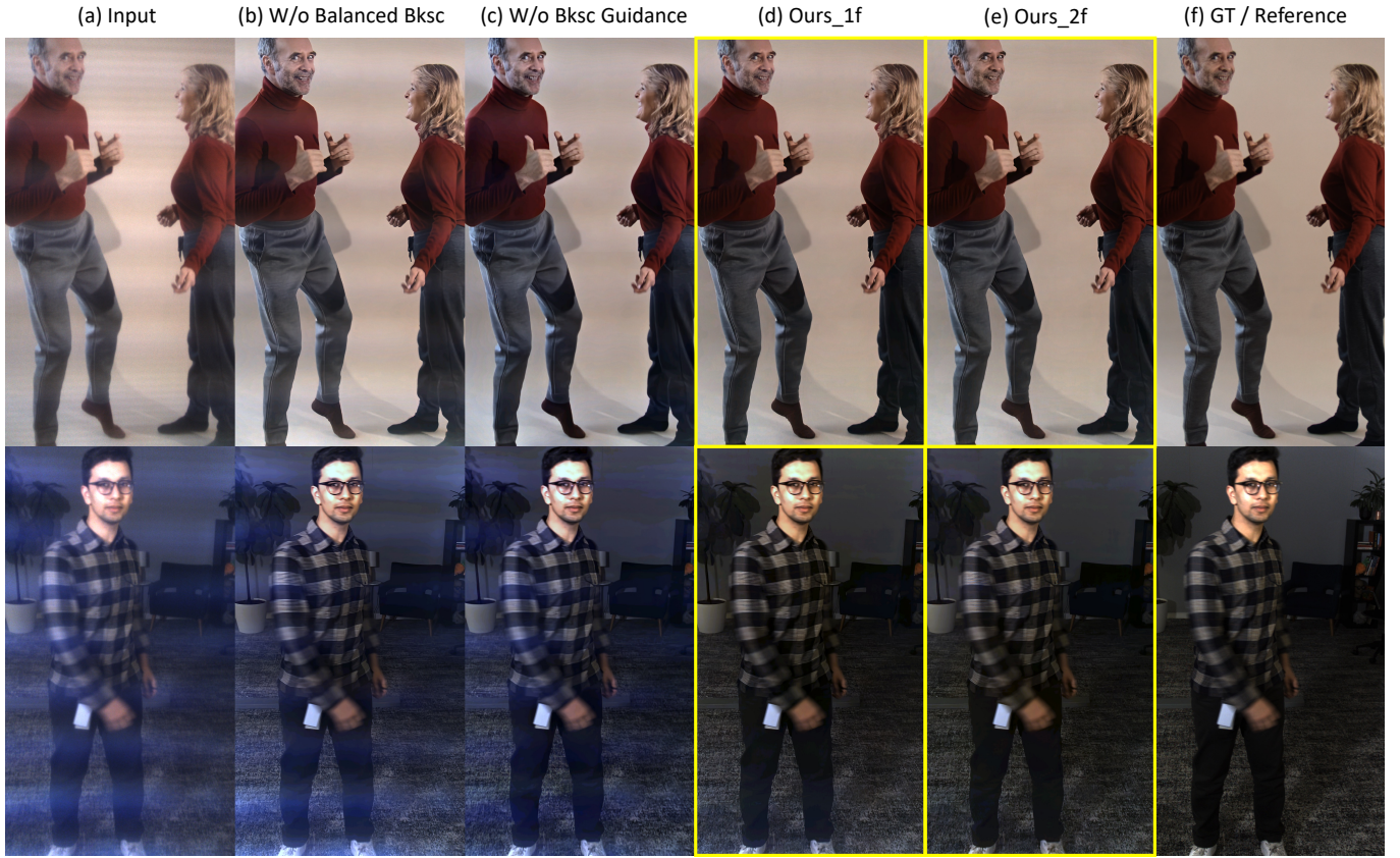
Fig. 12. Ablation study. The visual results show that a good training dataset with balanced backscatter simulations, the backscatter guidance in the network design, and previous frame as the input help improve the performance.
