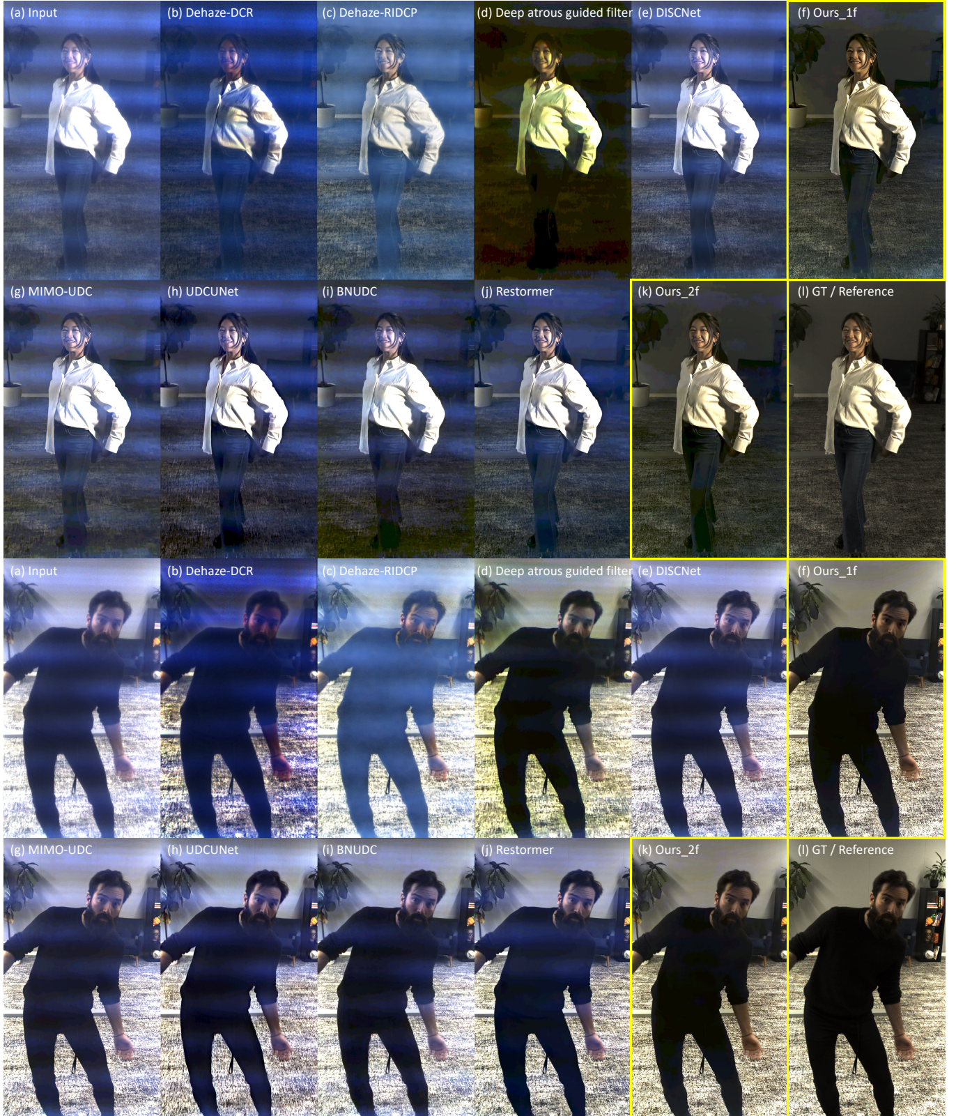
Fig. 11. Comparisons on real data Human-Real. Our method can remove backscatter and wire effectively while others cannot. Here, Ours_1f and Ours_2f refer to our methods using only the current frame and the current+previous frames, respectively.
